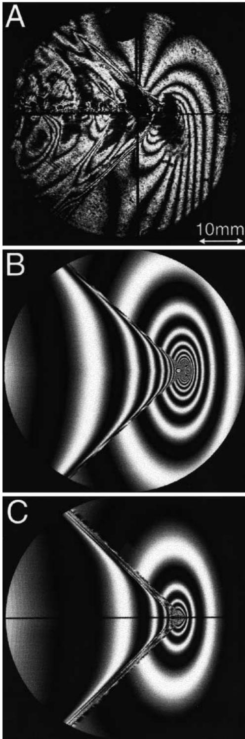
**Fig. 5** Enlarged view of the isochromatic fringe pattern around a steady state intersonic shear crack along a weak plane in Homalite-100. Shear shock waves are clearly visible. (A) Experimental Pattern, (B) Theoretical Prediction based on Freund's singular solution [14] and (C) Theoretical prediction based on a Dugdale type cohesive zone model by Samudrala et al. [22] (For all cases  $\beta=43^\circ$  and  $\nu=1.37 c_s$ )
