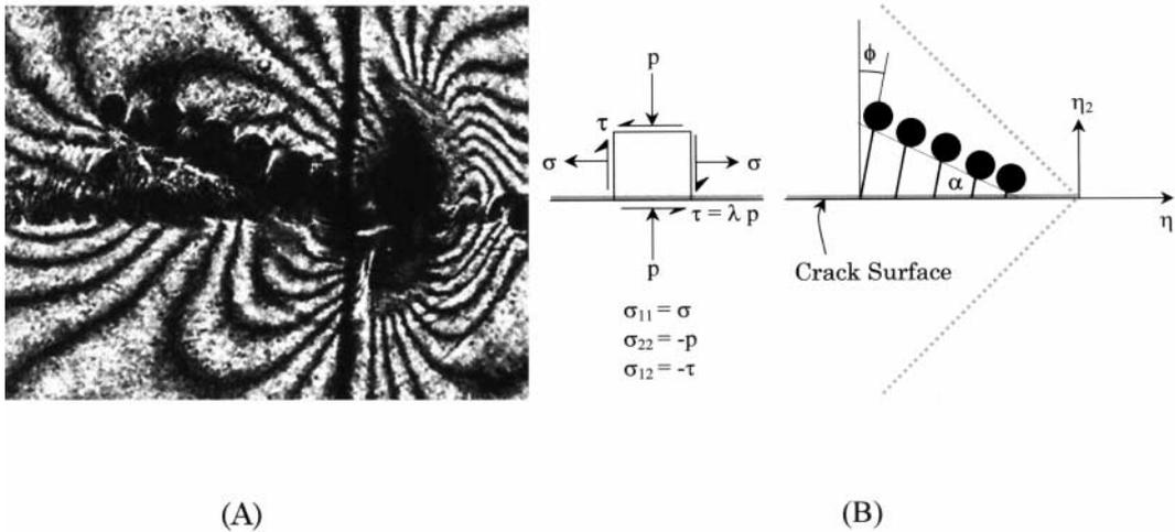
**Fig. 7.** (A) Enlarged view of the region behind the main intersonic shear crack tip showing the shadow spots associated with the subsonic secondary cracks originating from the contact zone. (B) Schematic showing the initiation and propagation of the tensile secondary cracks and the 2-D stress state on the contact face
